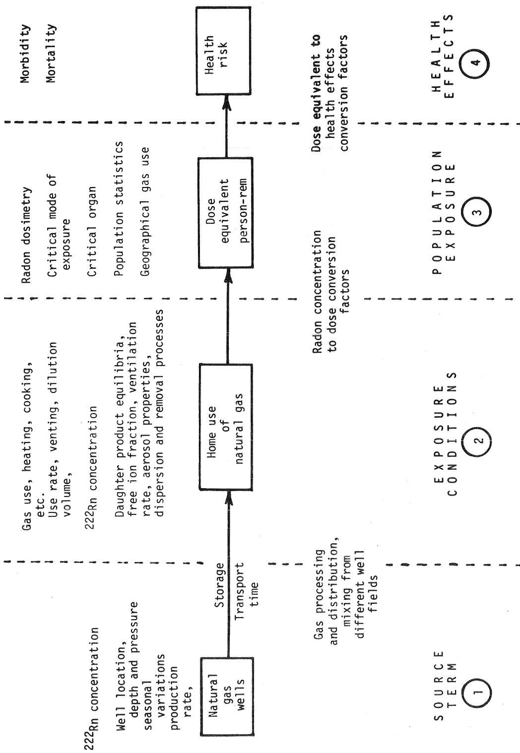
Figure 1. Model for estimating potential health effects from radon in natural gas
